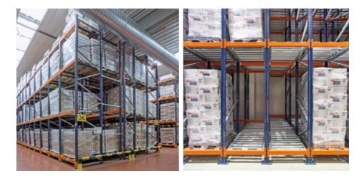
AGILITY AND SAFETY IN OPERATIONS: FORKLIFTS DO NOT HAVE TO ENTER THE RACKS AND ONLY WORK FROM ONE AISLE.
