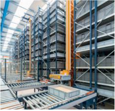
INTEGRATES THE RACKING, STACKER CRANE AND WAREHOUSE MANAGEMENT SYSTEM ROLLED INTO ONE.
