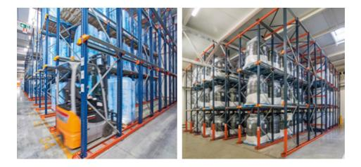
CAN BE USED WITH EITHER LIFO (LAST IN, FIRST OUT) OR FIFO (FIRST IN, FIRST OUT) WITH BATCHES WHEN THERE ARE MORE THAN THREE LANES PER SKU.
