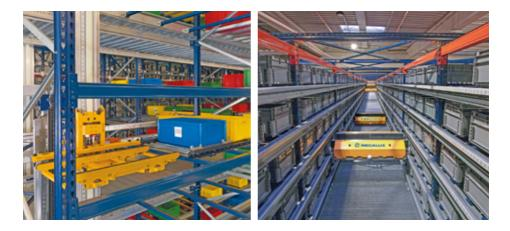
ADAPTABLE TO DIFFERENT UNIT LOADS: PLASTIC OR CARDBOARD BOXES AND METAL TRAYS OF MULTIPLE SIZES.
