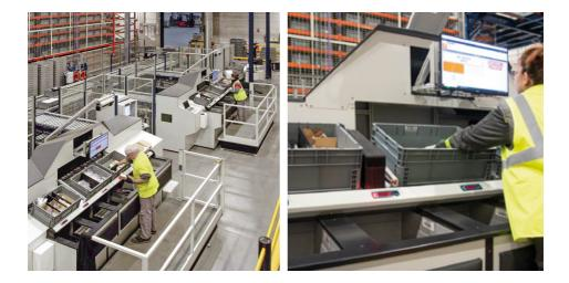
PICK-TO-LIGHT SYSTEMS STREAMLINE ORDER PICKING AND AVOID ERRORS DUE TO MANUAL HANDLING.
