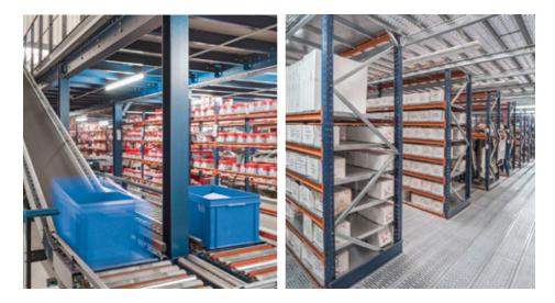
PICK MODULES CAN BE COMBINED WITH AUTOMATIC LIFTS OR CONVEYORS TO STREAMLINE MOVEMENTS BETWEEN LEVELS.
