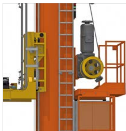
Hand ladder and top maintenance platform
