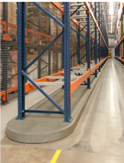
In mechanical guided aisle entry, profiles are fitted with reinforced entry rails to help centre the vehicles.
