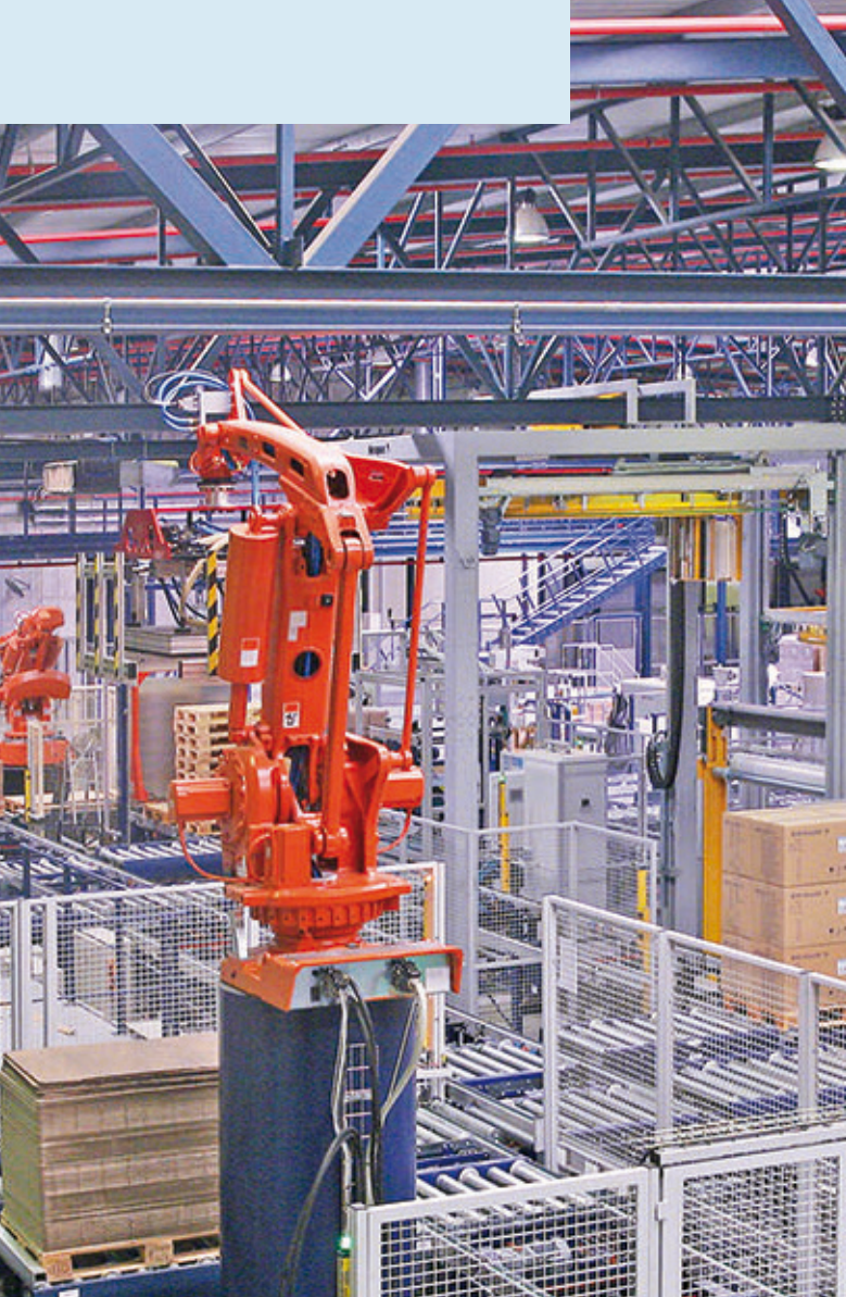
Automatic picking system depalletizer robot operation outline.
