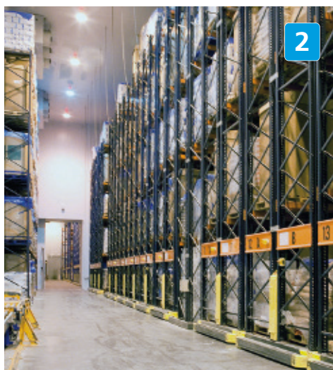
Half rotation orders or variable-sized pallets are stored on mobile bases.
