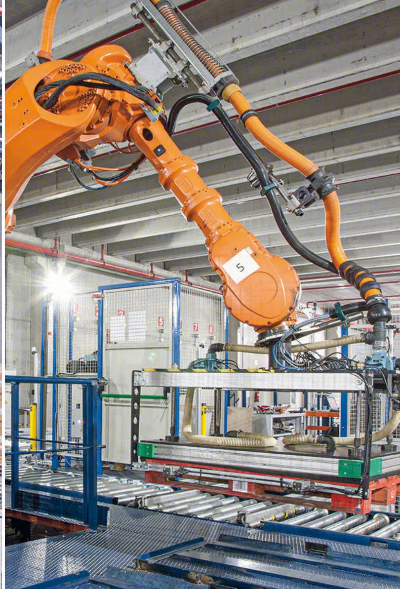
Automatic picking system depalletizer robot operation outline.
