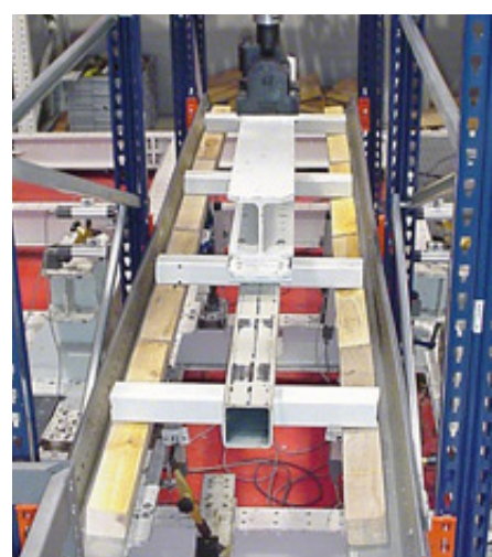
Figure 4. Example of a rail test for drive-in pallet racking.
